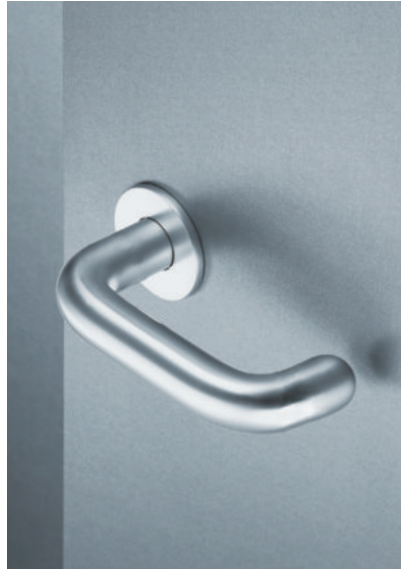
Modric 3506D Pair of 22øx133x67mm safety lever handles on 50øx3mm concealed Quadaxial fixing roses. Finishes: SS • PS • MA • TA • PB • PZ
